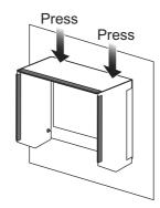
8. Set the hood assembly with the knobs tightly (4 pcs.).
